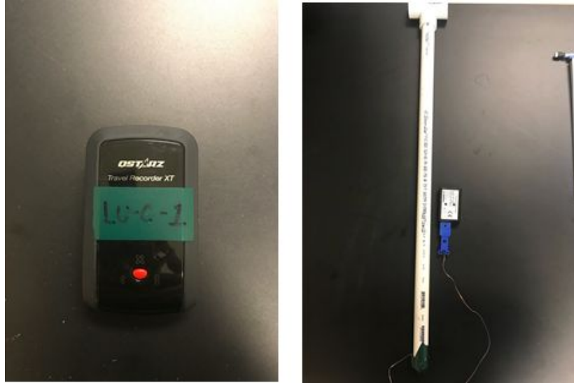
Figure 1. GPS tracking device (left) and thermocouple connected to data logger located inside a PVC pipe (right) (Austin et al. , 2019).
